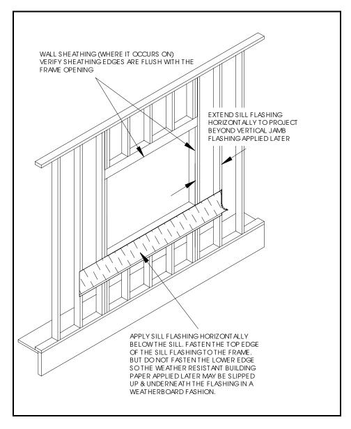
Figure 2: Sill Flashing
