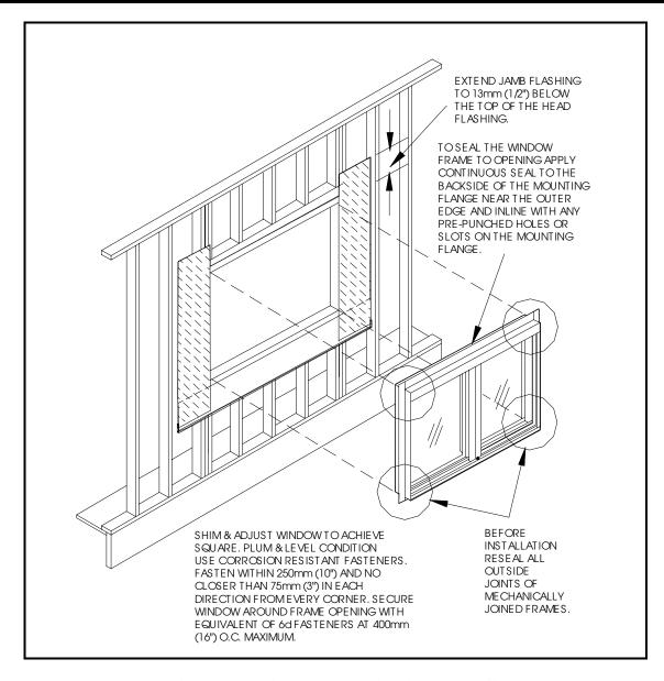
Figure 4B: Window Installation (Method "B")
