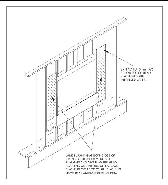
Figure 3B: Jamb Flashing (Method "B")
