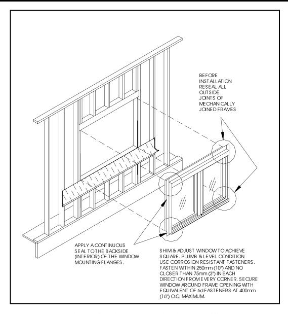
Figure 3A: Window Installation (Method "A")
