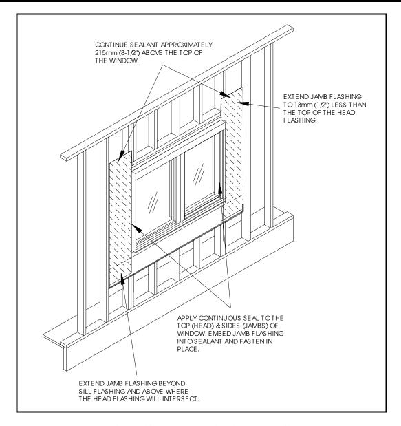
Figure 4A: Jamb Flashing (Method "A")
