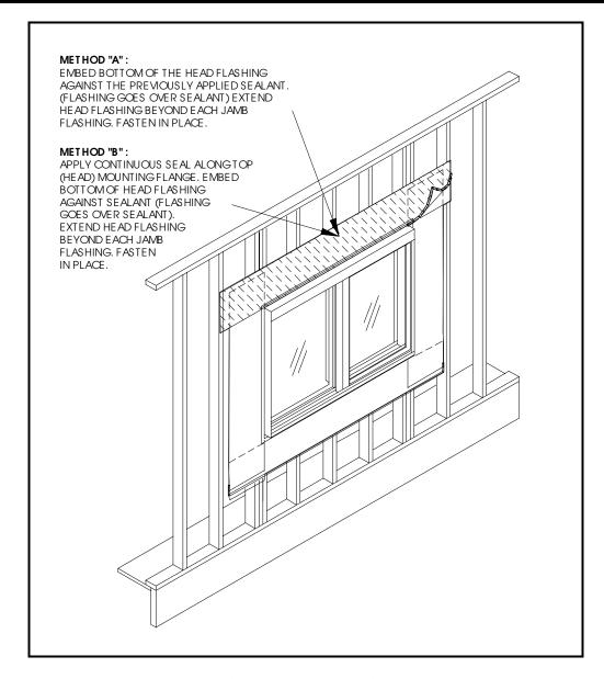
Figure 5: Head Flashing
