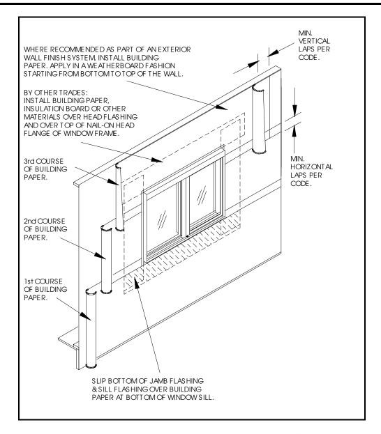
Figure 6: Primary Weather Barrier Application By Others
