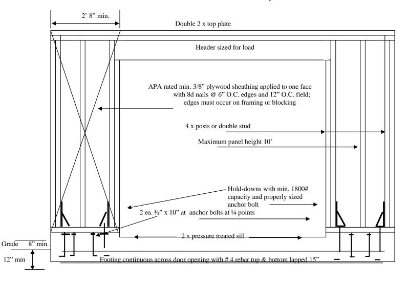
1<sup>st</sup> story of two story—plywood sheathing installed on both faces of each panel, 3 anchor bolts at 1/5 points and 3000# capacity hold down
